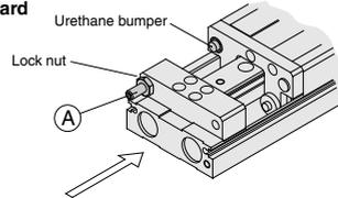
Loosen the stopper bolt lock nut on side (A), insert a wrench in the direction of the arrow to adjust the stroke, and then tighten the lock nut.
