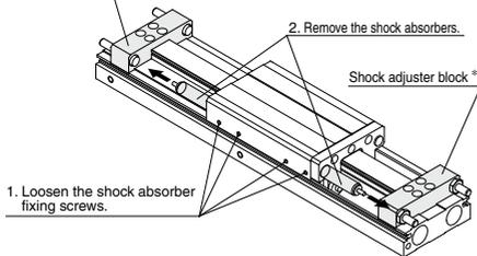
\* In the case of MXW8-25, first take out the adjuster block, and then the shock absorber. Tighten the mounting bolt with the torque 0.3 N·m when assembling the adjuster block.
