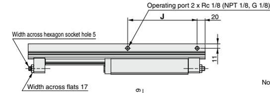
Note) If long bolts are used, they can touch the guide block and cause malfunction, etc. Refer to the Specific Product Precautions.
