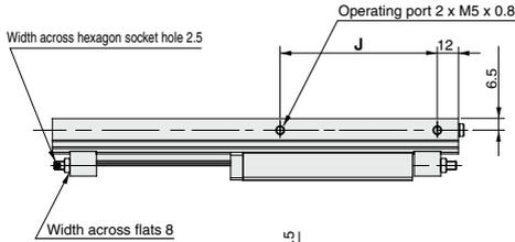
Note) If long bolts are used, they can touch the guide block and cause malfunction, etc. Refer to the Specific Product Precautions.
