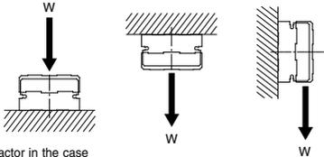
Note) No need to consider this load factor in the case of using perpendicularly in a vertical position.
