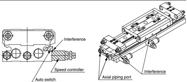
When an auto switch is installed on the port side of MXW8, some switches could interfere with the speed controller or a fitting. Therefore, use one of the methods described below for installing the auto switch.
