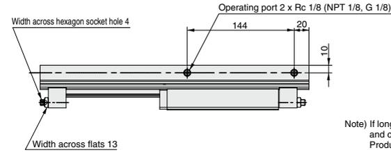
Note) If long bolts are used, they can touch the guide block and cause malfunction, etc. Refer to the Specific Product Precautions.
