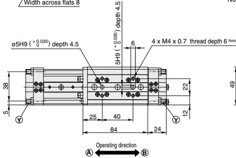
Note) If long bolts are used, they can touch the guide block and cause malfunction, etc. Refer to the Specific Product Precautions.
